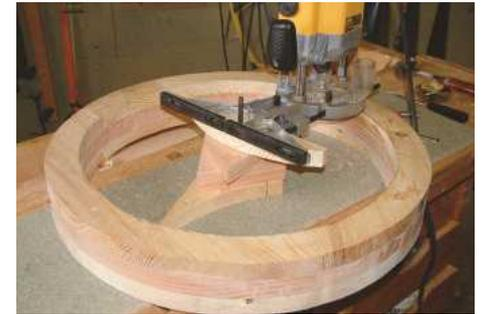
▲ Pic.10 Trim the inner and outer circumferences gradually with a long straight router bit
